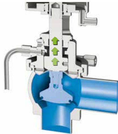
The aseptic barrier prevents the elevator effect
