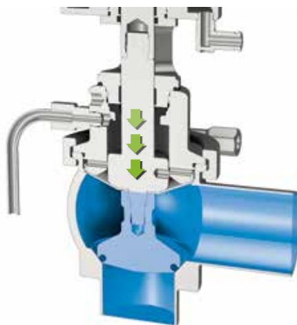
The aseptic barrier prevents the shuttle effect
